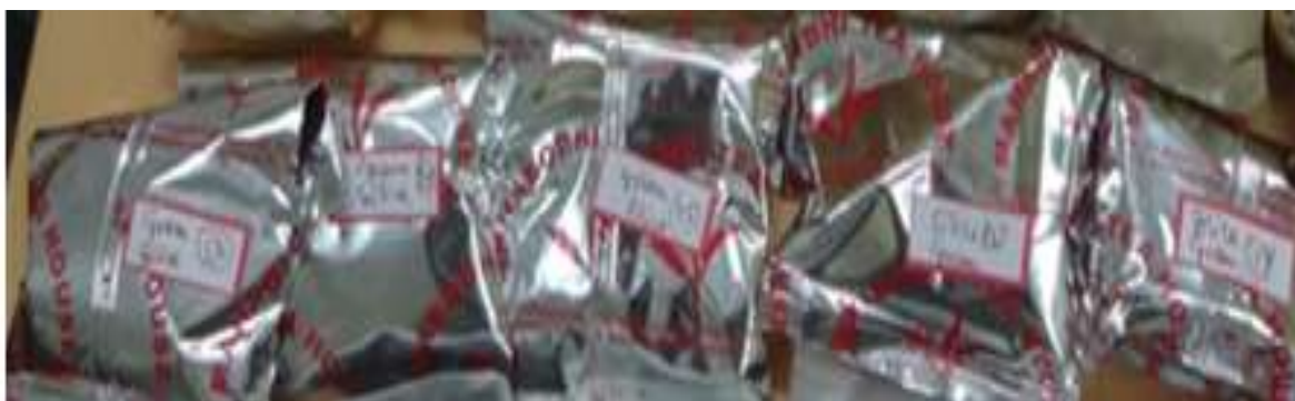
Figure 3.19: Shows that the manufactured tea are stored in Aluminium packaging with silica desiccants
