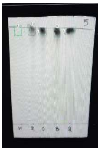
Figure 4.5.11.1a Thin-layer Chromatography of manufactured tea with Iron Chloride-Ethanol reagent coloring agent and with standard Quercetin.
