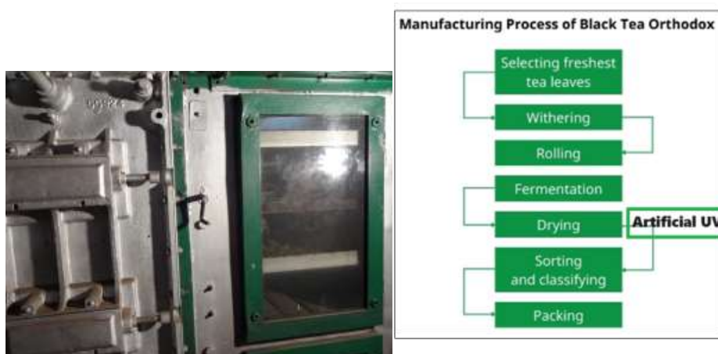
Figure 4.4.12.1: Factory set up of artificial UV lamp
